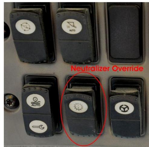
The RPM should go back from 2100 to approximately 1700 RPM and recover within one second up to 1950-1980 RPM. The machine should of course not move. As mentioned above these values are valid only for CAT® 966G. But most wheel loaders have more or less similar values.
